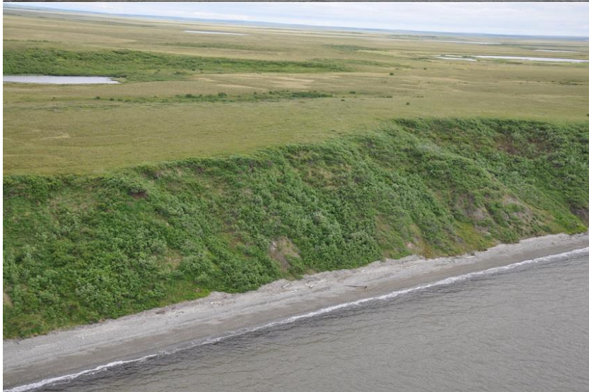
Figure 1c. Stability Class CE2 , an actively eroding, completely vegetated cliff (>90% vegetation cover) but with "disturbed vegetation (indicating down-slope movement)
