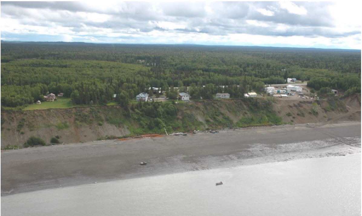
Figure 12. Oblique photo of rapidly eroding cliff in Cook Inlet. A pickup truck is on the lower portion of the beach. The cliff height is approximately 30m and the beach width is approximately 50m.
