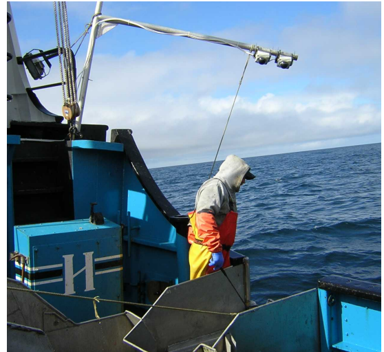
Figure 2. Video monitoring equipment (on stanchion above the crew member) is used to record the species caught.
