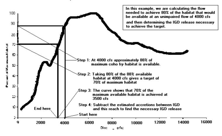
**Figure 8**. Example of method used to determine necessary flow release from IGD to achieve a target of 80% or 90% of maximum habitat available at a given unimpaired flow in the Shasta to Scott river reach.
