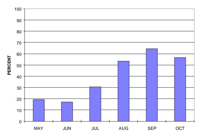
**Figure 3**. Monthly average Iron Gate Dam contributions to Klamath River flows measured at Orleans (1962-1991). Data are from Hydrosphere Data Products, Inc. (1993).
