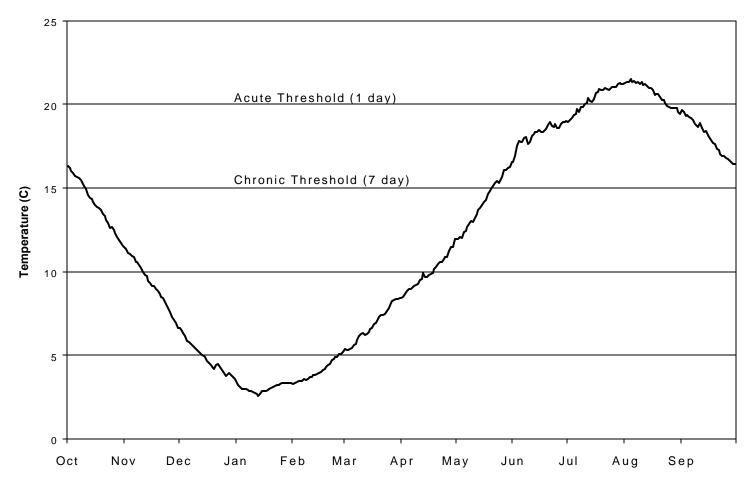
**Figure 6**. Average daily maximum water temperatures in the Klamath River below Iron Gate Dam (1963-1979). Acute and chronic high temperature thresholds are 1986 Environmental Protection Agency criteria (Campbell 1995). Data are from Hydrosphere Data Products, Inc (1993).
