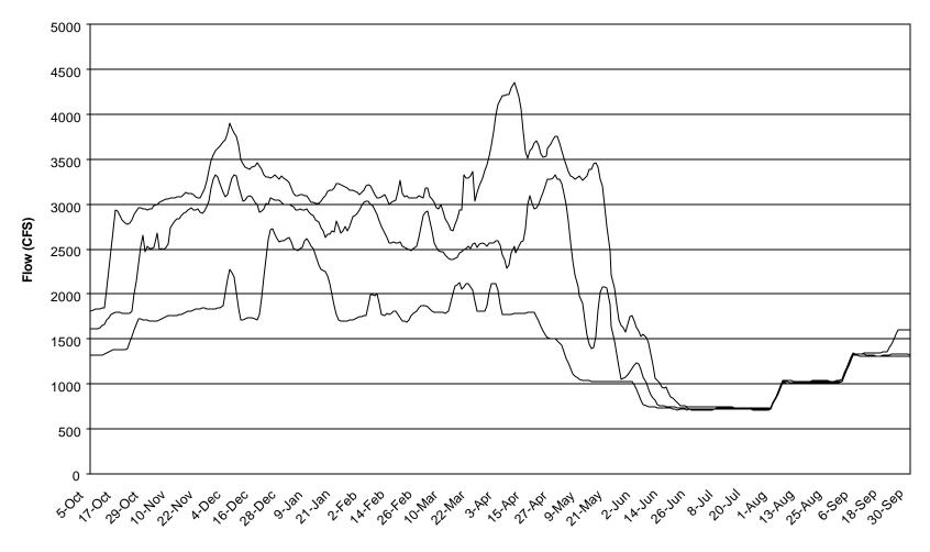
**Figure 1**. Average Klamath River flow at Iron Gate Dam, California - Normal water year median, 25th and 75th percentile (1963, 1966, 1969, 1970, 1973, 1985, 1989; 5 day moving average). Data are from Hydroshere Data Products, Inc. (1993).
