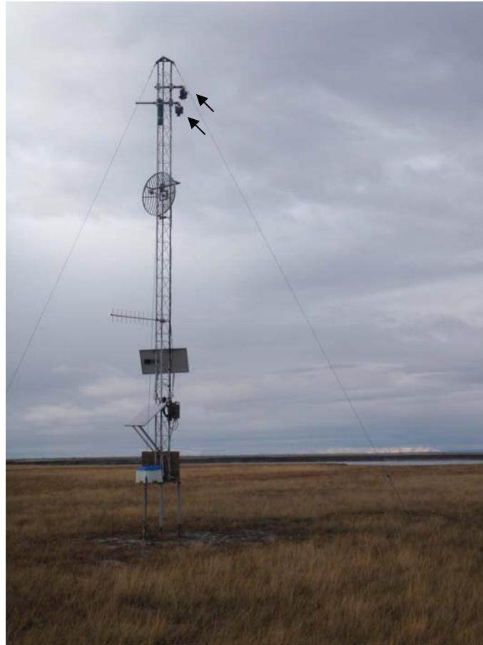
Figure 3: Camera tower with two cameras mounted near the top, arrows pointing towards cameras.
