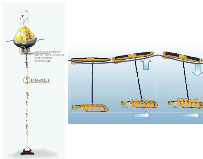
Figure 9. Schematic of PRAWLER mooring which profiles the upper water column and Wave Glider (CWG & EWG; NOAA-PMEL) which is a remotely controlled autonomous vehicle consisting of a surfboard-like surface float with solar panels to power communications and instrumentation. The two wave gliders were outfitted with different sensors (carbon and ecosystem).
