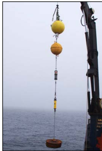
Figure 11. Oceanographic current meter mooring being deployed.
