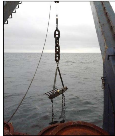
Figure 35. Dragging rake and hooks being lowered through the A-frame.
