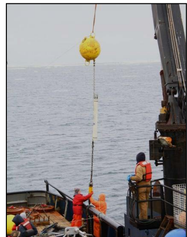
Figure 2. Long-term passive acoustic mooring being retrieved.
