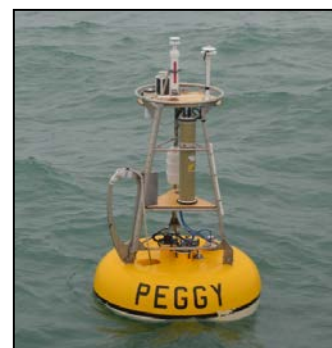
Figure 14. Oceanographic mooring with surface float.
