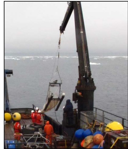
Figure 20. Tucker sled being deployed around ice.
