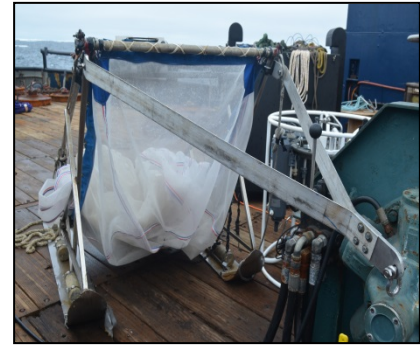
Figure 19. Tucker sled with the custom bridal to prevent the wire from twisting.
