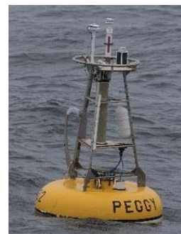
Figure 14. Oceanographic mooring (M2) with surface float.
