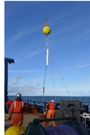
Figure 2. Long-term passive acoustic mooring being deployed.
