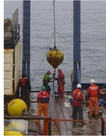
Figure 24. Successful dragging attempt and retrieval of mooring through A-frame.
