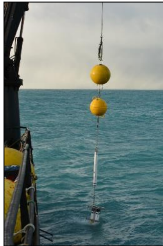
Figure 11. Oceanographic ADCP mooring being deployed.
