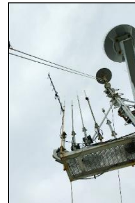
Figure 7. Sonobuoy antennas placed in the crow's nest (far left mast).
