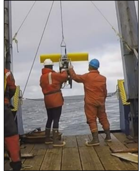
Figure 18. Acrobat towfish being deployed.
