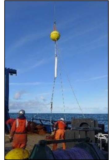
Figure 2. Long-term passive acoustic mooring being deployed.
