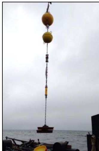
Figure 11. Oceanographic ADCP mooring being deployed.
