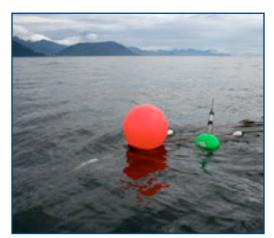
Telemetry buoy, housing a GPS transmitter, tracks an entangled whale. The buoy is attached to the gear entangling the animal.
