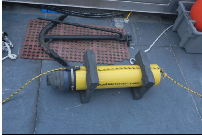
Figure 7. Rigging of the Autonomous Data Recorder in Moored Configuration.
