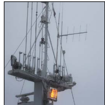
Figure 7. Sonobuoy antennas placed in the crow's nest.
