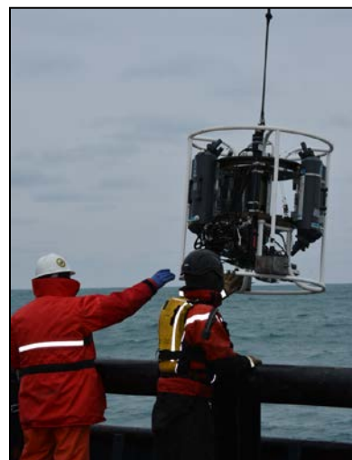
Figure 15. CTD being deployed.
