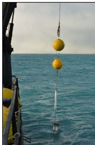
Figure 11. Oceanographic ADCP mooring being deployed.
