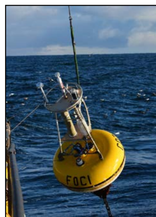
Figure 14. Oceanographic mooring with surface float.
