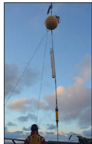
Figure 2. Long-term passive acoustic mooring being deployed.
