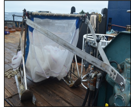
Figure 17. Tucker sled with the custom bridal to prevent the wire from twisting.
