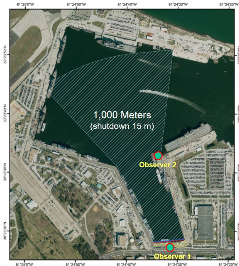
Figure 1. Positions of the observers during in-water pile driving.
