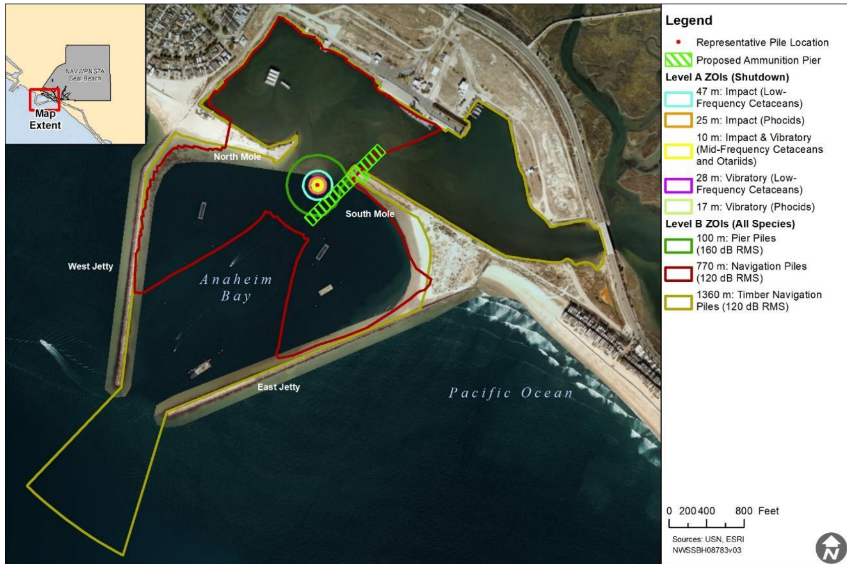
Figure 2: Underwater Sound Zones of Influence for Pile Activities at the New Pier (24-inch concrete and 16-inch concrete filled fiberglass piles) and Existing Navigation Piles (24-inch timber and steel pipe piles)
