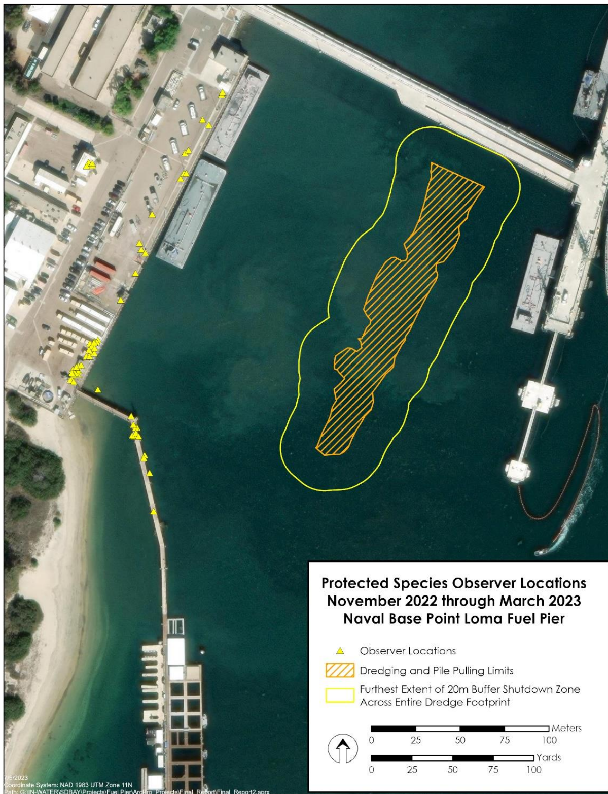
Figure 1. Project Area and Locations of Protected Species Observers during In-water Activities (November 2022–March 2023).
