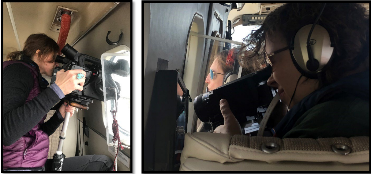
Figure 4. -- Video cameras and setup used during the 2021 (left) and 2022 (right) Cook Inlet beluga aerial survey. In 2021, a Sony HXR-NX5U HD video camera (1920 × 1080 pixel resolution) was paired with a “zoomed” Panasonic HC-X1 (3840 × 2160 pixel resolution) (left) while in 2022, two 4K Sony FDR-AX700 video Handycams (3840 × 2160 pixel resolution) replaced the larger video cameras (right).
