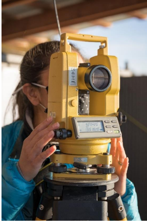
Photo 13. PSO using Topcon DT-205 digital theodolite (Photo Credit: Kristina Smolenski – The Photo Gecko)
