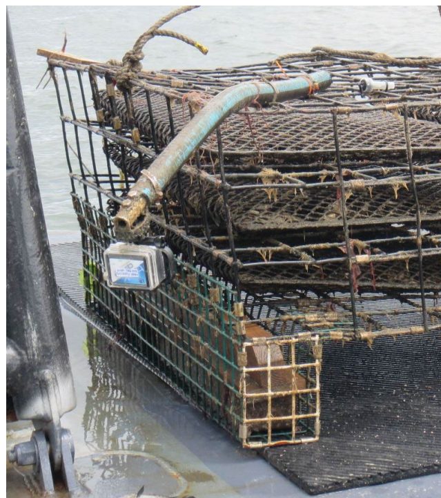
Photo above shows camera mounted to the corner of the oyster cage using flex marine wet exhaust water hose
