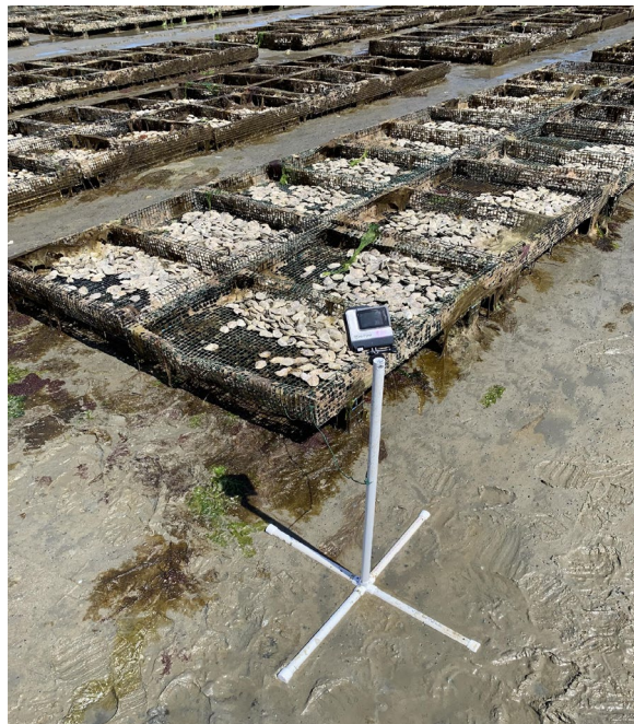
Photo above shows PVC mounting stands for cameras placed adjacent to oyster trays.
