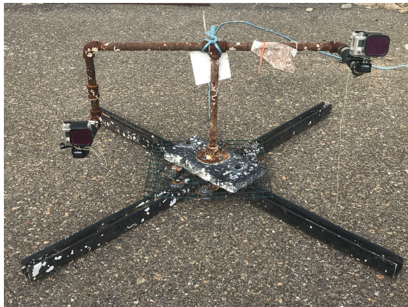
Photo above shows T-platform base for mounting cameras adjacent to boulders on the seafloor
