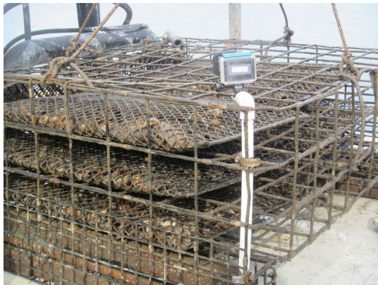
Photo above shows the periscope style mount used to view across top of oyster cages
