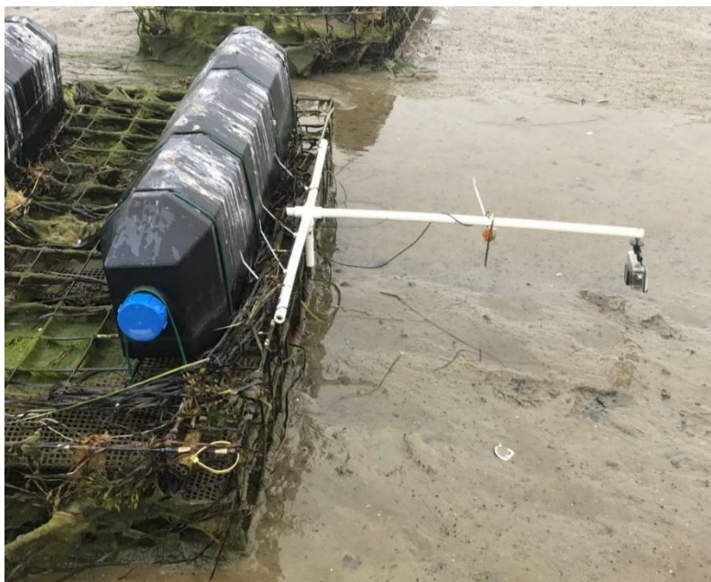
Photo above shows camera mount for floating cage
