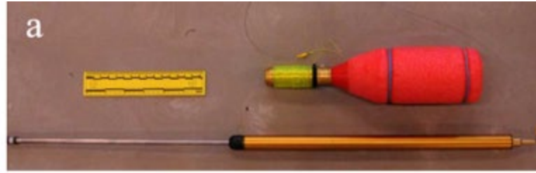
Figure 14. Paxarms whale dart (bottom) and tether and float (top) from Moore et al. 2013
