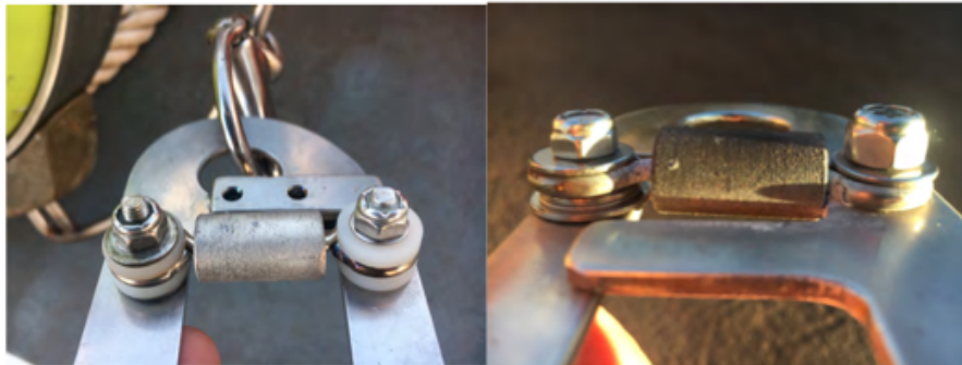
A new galvanic release isolated from the clip. A burnished, un-isolated release
