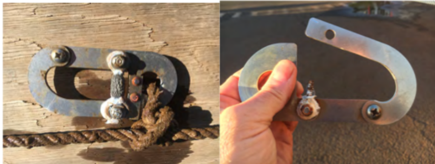
A pitted galvanic release in need of replacement and a spent timed release in need of a new galvanic release. Not the missing hardware on the open clip side.
